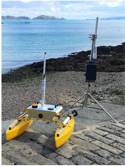
The Marine Electronics Autonomous Survey Vessel (ASV) is designed for remote bathymetric surveying of lakes, ponds, reservoirs, canals, rivers etc using a number of different sonar devices with real time display using a wireless LAN with up to 3km range.
